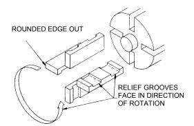
Figure 4 - Vane Installation
