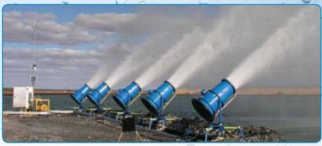
Due to new regulations, Australian mine operators can no longer discharge water into nearby waterways. Today, the most efficient and effective way to eliminate this water is through an evaporation process.
